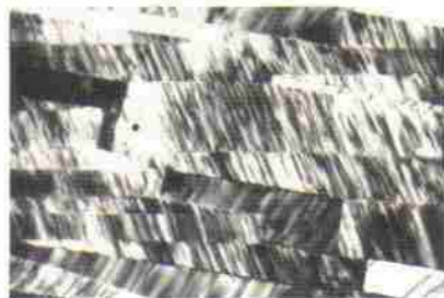
Fig. 9 (left). High resolution electron microscopy image showing periodic stacking faults inside martensite variant in \text{Ni}_{46.8}\text{Mn}_{48.5}\text{Ti}_{5.0} .
